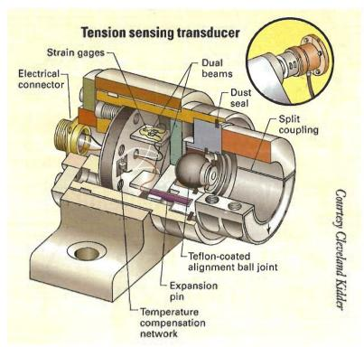
The transducer is first fastened to the machine frame at one end and to a roller on the other end. Then, the web is wrapped over the roller. Inside each transducer, strain gages have been attached to a pair of beams made of spring steel.
