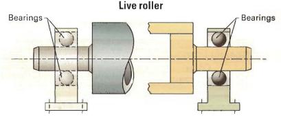
Rotating shaft rollers are designed so that the entire shaft is part of the spinning assembly.
