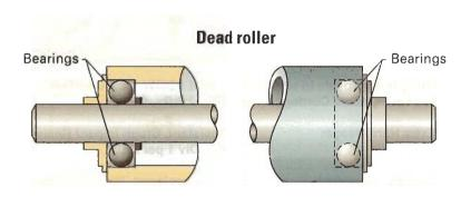
On stationary rollers, the shaft stays put while an outer sleeve rotates around the shaft on bearings.
