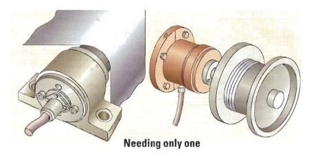
Left: On narrow webs, rollers are typically cantilevered — and the setup requires only one load cell. Right: Lines that spool wire or cable often run over pulleys. Again, only one cell (at the support) is needed.
