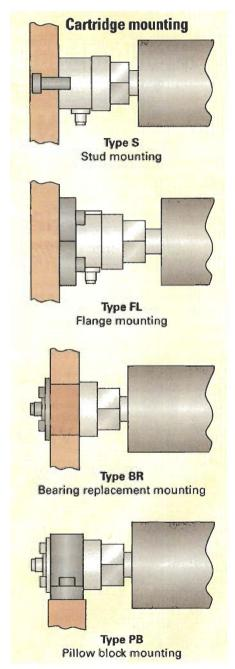
Cartridge-style load cells can be mounted in a number of ways, making them convenient for a myriad of applications.
